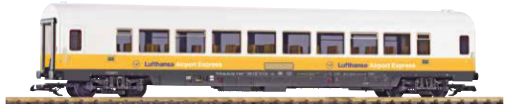
37668 Personenwagen Bpmz 296 Lufthansa DB Ep. IV Passenger Car Coach Bpmz 296 Lufthansa DB IV
